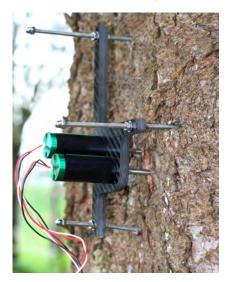
**Displacement transducer:** Weatherproof but not sealed potentiometer for measuring in a  $\mu$ m resolution. Hub of the moving rod is 2 cm.
