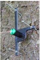
Voltage-Sensitivity: 1 mV =  $4.0 \mu m$ Temperature-Sensitivity:  $< -0.28 \mu m °C^{-1}$
